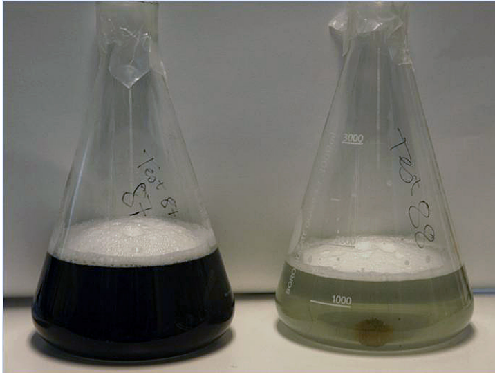
Figure 5.3 Water collected after cleaning of the polyethylene sheet. The two bottles are from two different ammunitions.
